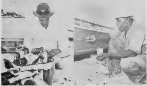
A CLOSE inspection of the motor is good insurance before starting out. Any loose calking should also be replaced. An important piece of survival equipment is an anchor, left, and plenty of line. If the motor should fail, the anchor keeps the boat from drifting with the current and improves chances for rescue.
